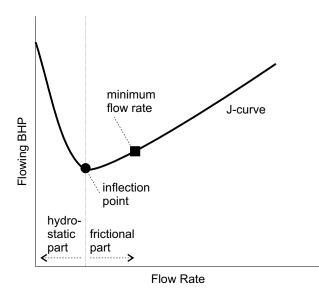
The J-curve is divided into two parts by the inflection (loading) point, where the slope is zero. To the left is the hydrostatic contribution. To the right is the contribution from tubing frictional losses. The minimum flow rate corresponding to the minimum velocity (as determined by the 10 ft/ sec. rule of thumb or the Turner *et. al.* (1969) correlation) also appears on the J-curve.
