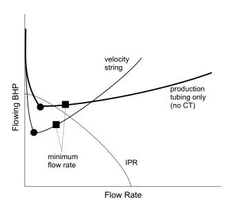
It is also important to make sure the velocity string design will keep the well flowing long enough to recoup the cost of the installation, as the reservoir pressure continues to drop. To see the future performance of the velocity string, create the IPR for the predicted future reservoir pressure and compare it with the J-curve of the velocity string. Make sure that the actual flow rate at the future pressure is still greater than the minimum flow rate.
