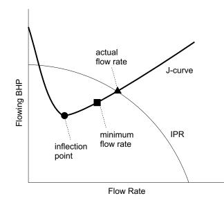
If the intersection point is between the inflection point and the minimum gas flow rate, liquid loading occurs. The well flows, but will eventually kill itself.
