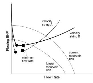
If multiple designs will prevent the well from loading up, the optimum choice is typically a trade-off between current production (a higher flow rate) and sustained production (a lower bottomhole pressure).
