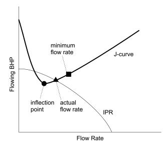
If the IPR and J-curve do not intersect, or if they intersect to the left of the inflection point, the flowing bottomhole pressure is too low for the well to flow for that particular tubing size, depth, and wellhead pressure. You should consider another velocity string design.
