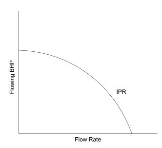
There are various methods available in the literature to construct the reservoir IPR for oil and gas wells. Cerberus constructs the reservoir IPR based on Darcy's equation for oil wells. This can be somewhat of a limitation since many velocity strings are installed in gas wells with high gas-liquid ratios (GLRs).
