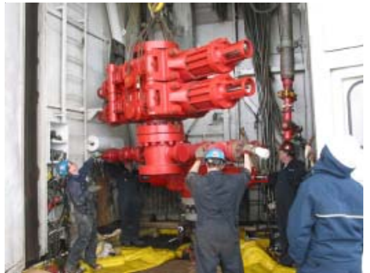
Fig. 3 Handling of 13 5/8" BOP
