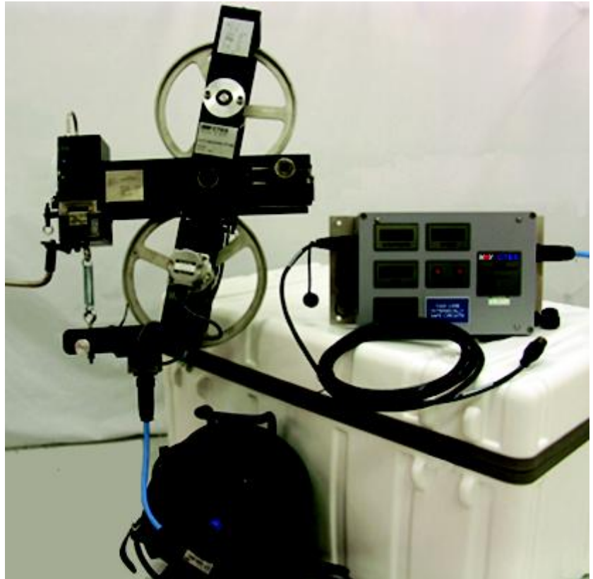
The DMS is a precision measuring instrument. It is designed to be quickly and easily installed or removed from the CT prior to transport. A padded storage box is provided for DMS transport and storage.
